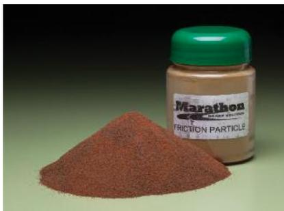
Rubber and friction particle, along with graphite, are part of a second tier of raw materials from an importance/cost perspective. Rubber, typically recycled tire treads, and friction particle derived from cashew shells are both organic materials that help to make the friction softer and more compressible.
