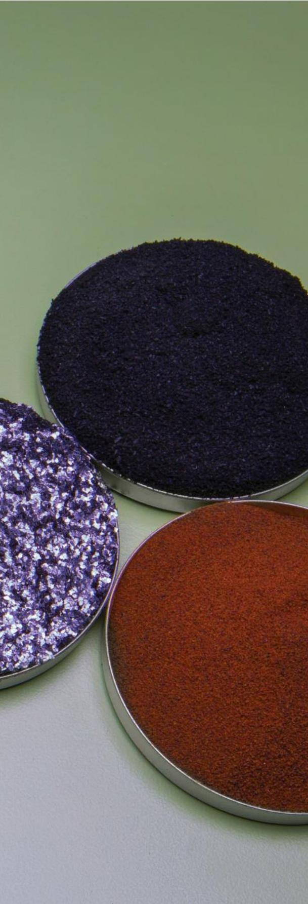
Graphite is also an important raw material, as it is temperature resistant and acts as a lubricant for the lining, thus greatly aiding in reducing wear and stabilizing friction level. Because different types of graphite exhibit varied frictional characteristics, many combinations or forms of graphite may be used in a friction formula based on the application of the lining.
